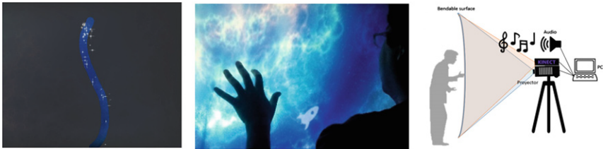
Fig. 3. The BendableSound prototype. A screenshot of the Level 1 of the BendableSound prototype (left). A user interacting with the fabric-based surface moving elements in the space (center). A mockup representation showing the hardware installation of the BendableSound prototype (right).
