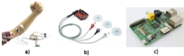
Fig. 4. Hardware utilized. (a) Positioning of the electrodes (b) Arduino plate with EKG/EMG Shield and (c) RaspBerry Pi
