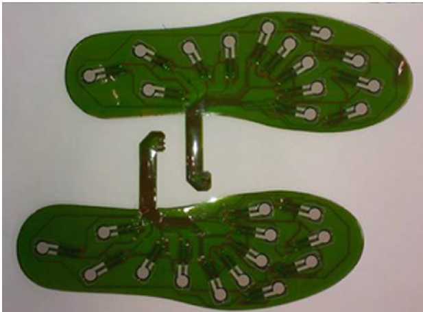
Fig. 2. Pressure sensor layer of the insoles
