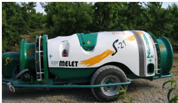
Fig. 2 Air-assisted sprayer with two axial fans with reverse rotation
