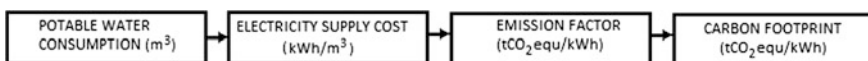
Fig. 2 Methodological scheme for the calculation of the carbon footprint of a potable water supply
