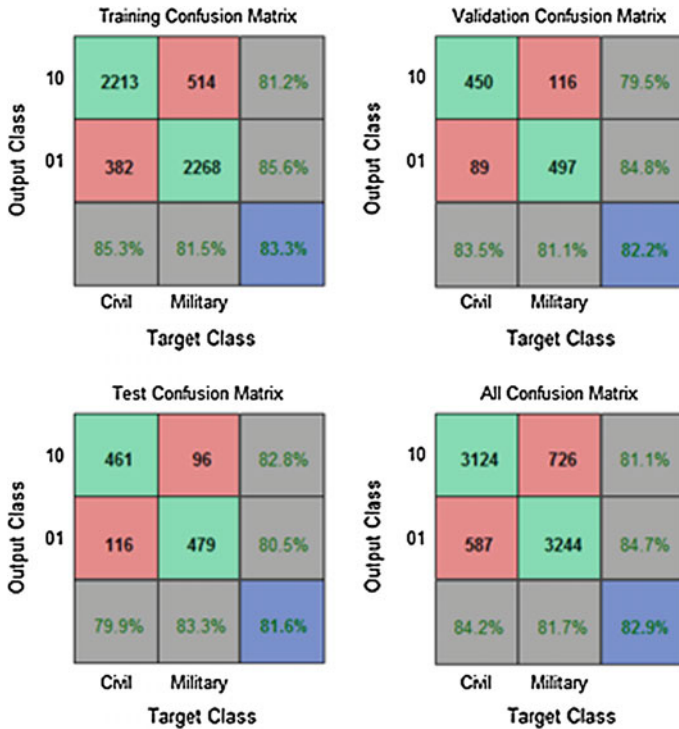
Fig. 5 Classification results for 12-10-2 NN classifier with normalised input data and a validation stop after 118 epochs. The values in green specify the correctly classified samples for each class (10—Civil, 01—Military)
