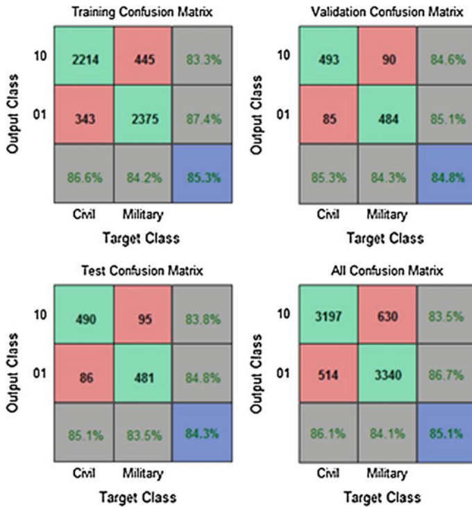
Fig. 6 Classification results for 22-22-2 NN classifier with normalised input data and a validation stop after 114 epochs. The values in green specify the correctly classified samples for each class (10—“Civil”, 01—“Military”)
