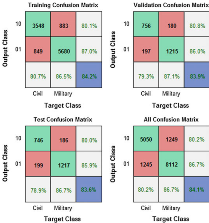
Fig. 8 Classification results for imputed data case for 12-10-2 NN classifier with normalised input data and a validation stop after 106 epochs. The values in green specify the correctly classified samples for each class (10—“Civil”, 01—“Military”)
