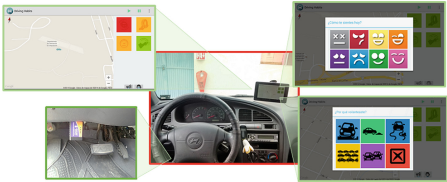
Fig. 1. The driving habits system. Upper left, the application main screen, Bottom left, the ELM327 device plugged into the vehicle OBD-II port, center, the android device running the application mounted over the dashboard, Upper right, the emotion status survey, Bottom right, the aggressive behavior event survey.
