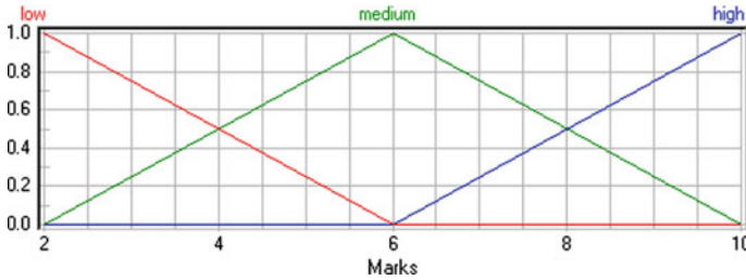
Fig. 2 Fuzzification of an input variable using three triangles as membership functions (mf)
