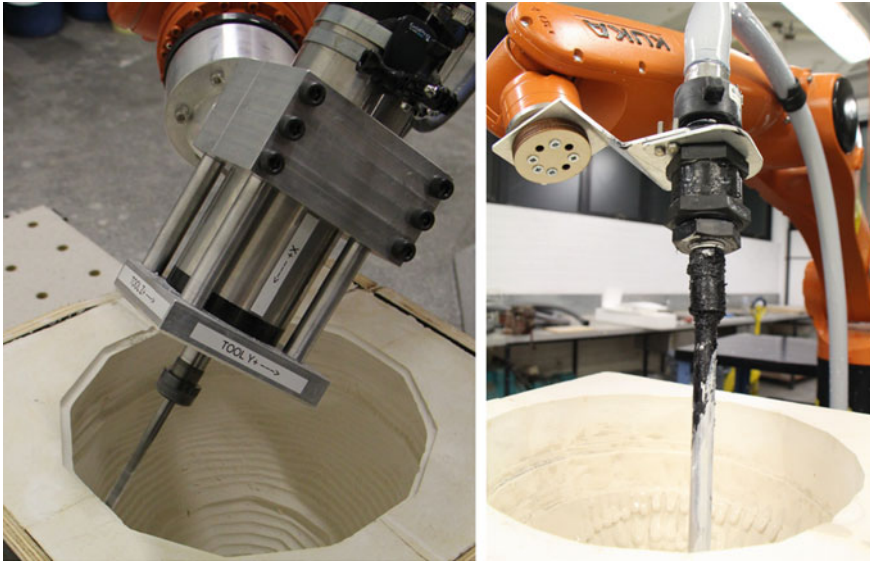
Fig. 1 Plaster Milling for Slip Cast mold ( left ), and clay deposition ( right )
