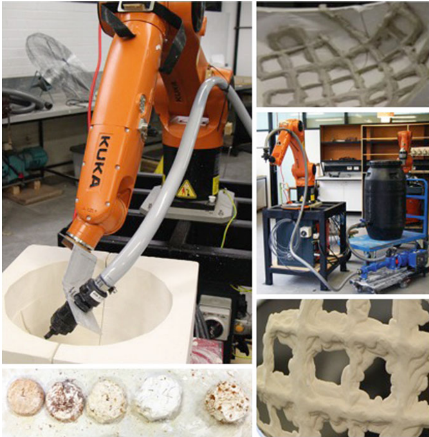
Fig. 3 Robotic work envelope, material storage and accessibility, flow of clay depending on viscosity and speed of the pump and raw and fired test samples
