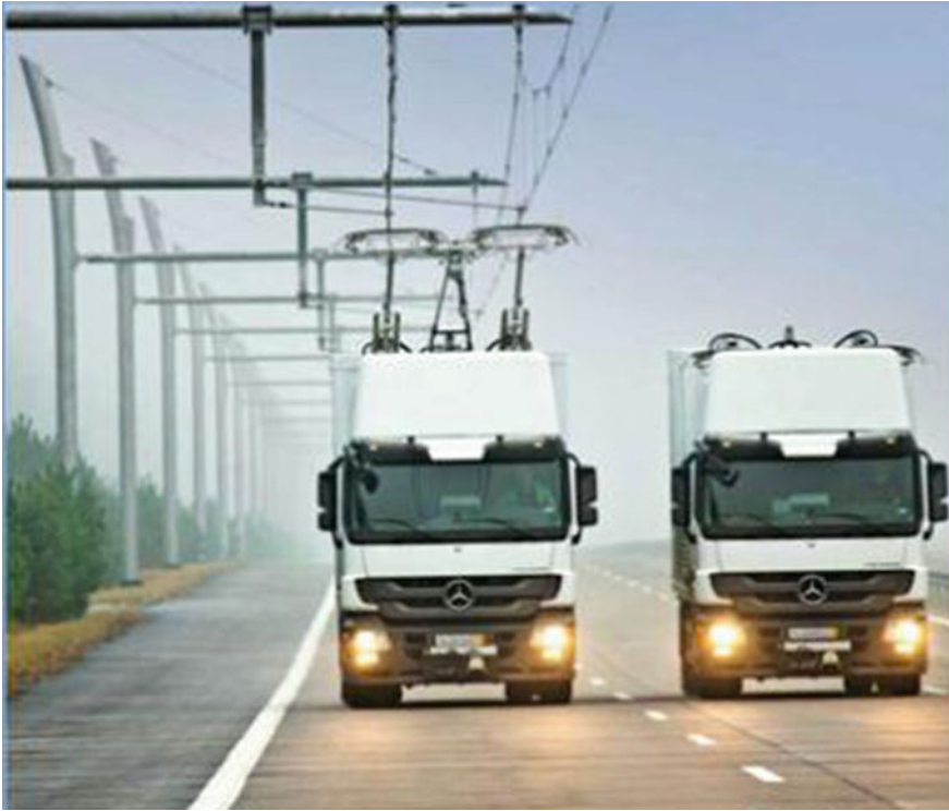
Fig. 14.1 I-710 Siemens demonstration project with one mile catenary system. Cost $13,500,000. Source AQMD (2015)
