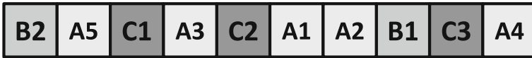
Fig. 1. OLE Fragmentation: The order of blocks in data streams is randomized, fragmenting the payloads
