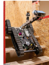
Fig. 3. Robot climbing stairs
