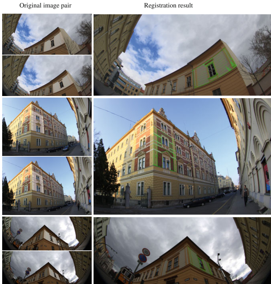
Fig. 6.10 Homography estimation results on real omni image pairs. Segmented regions are overlaid in lighter color, while the result is shown as the transformed green contours from the first image region over the second image
