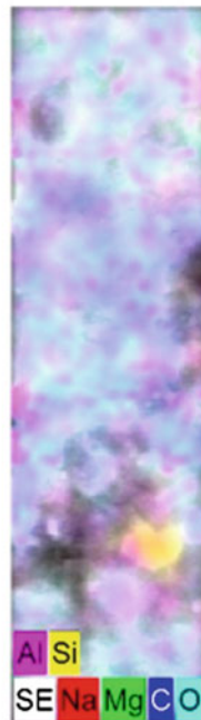
Fig. 26.5 Color image of Al_2MgSiO_4 compound at the interface
