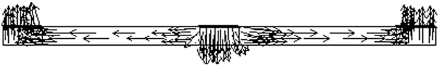
Fig. 46.2 Non-uniform polarization of ceramic layer
