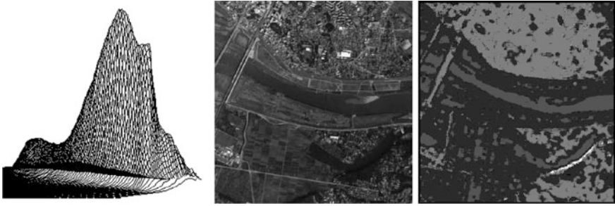
Fig. 19.5 Left Histogram of (\alpha_{\min}, \alpha_{\max}) related to the aerial photograph of Toride. Middle and Right Original and segmented aerial photograph of Toride
