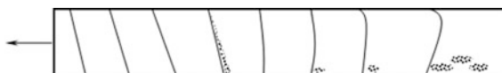
Fig. 8.2 Scheme of position of the crystallization front and excess of bubbles at various stages of crystal growth (the arrow shows the direction of crucible movement)
