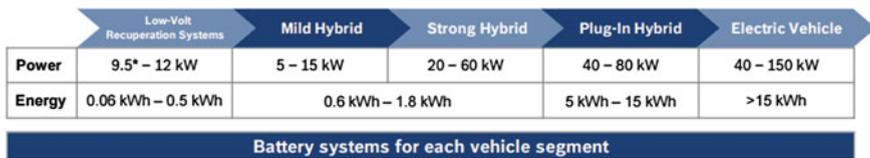
**Fig. 38** Overview of different battery systems by Bosch [42]
