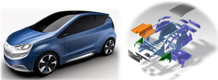
**Fig. 98** CULT, vehicle (*left*) and explosion view (*right*) [113]
