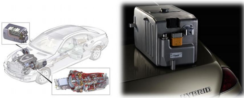
**Fig. 20** Daimler Mild-S400 BlueHYBRID with Li-ion battery pack [22]
