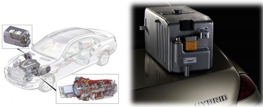
Fig. 20 Daimler Mild-S400 BlueHYBRID with Li-ion battery pack [22]
