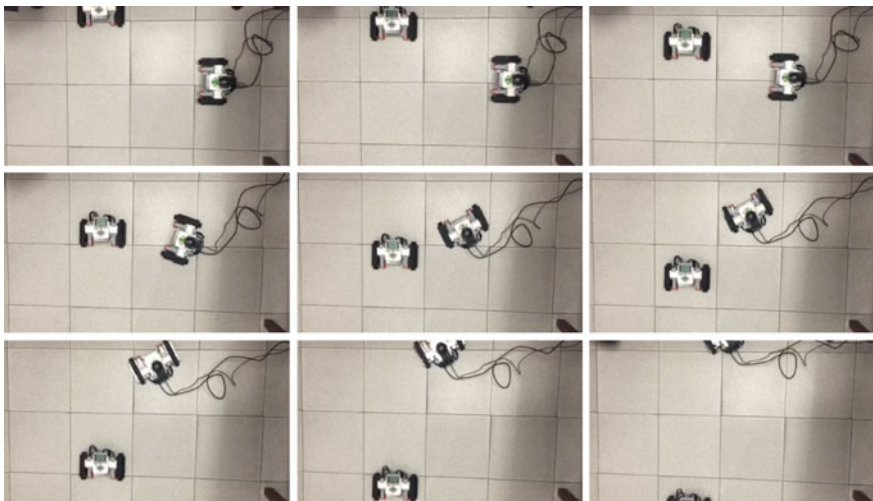
Fig. 20 Image sequence of the trajectory of robot for the right turn action
