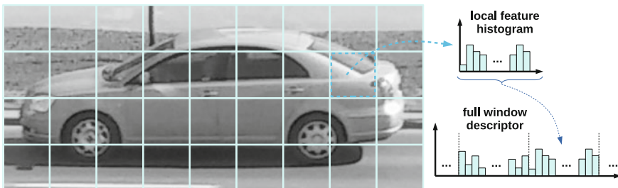
Fig. 1 The illustration of complete window descriptor formation based on local feature histograms
