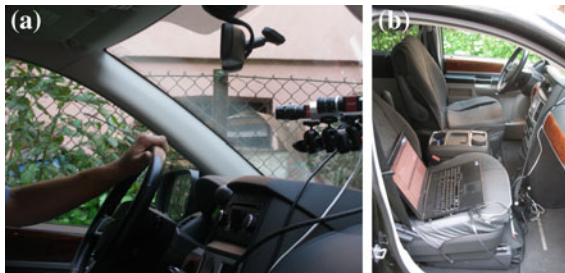
Fig. 2 Views of the driver's eye recognition system mounted in a car
