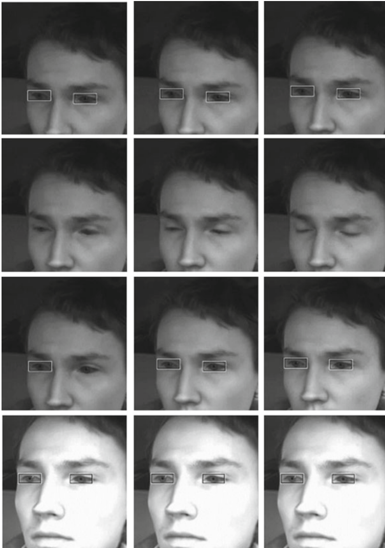
Fig. 3 Exemplary frames of driver's eye tracking in the NIR images in night conditions
