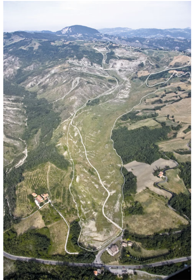
Fig. 18.8 The Ca' Lita landslide, reactivated in 2002 and 2004 (Reggio Emilia Province, photo G. Bertolini, 2012). During the 2004 event the landslide toe advanced for more than 400 m, filling a previously existing gully (Borgatti et al. 2006; Corsini et al. 2009). The activity of this landslide is probably co-determined by the inflow of highly mineralized groundwater mixed with methane uprising along a regional fault line (Cervi et al. 2012)
