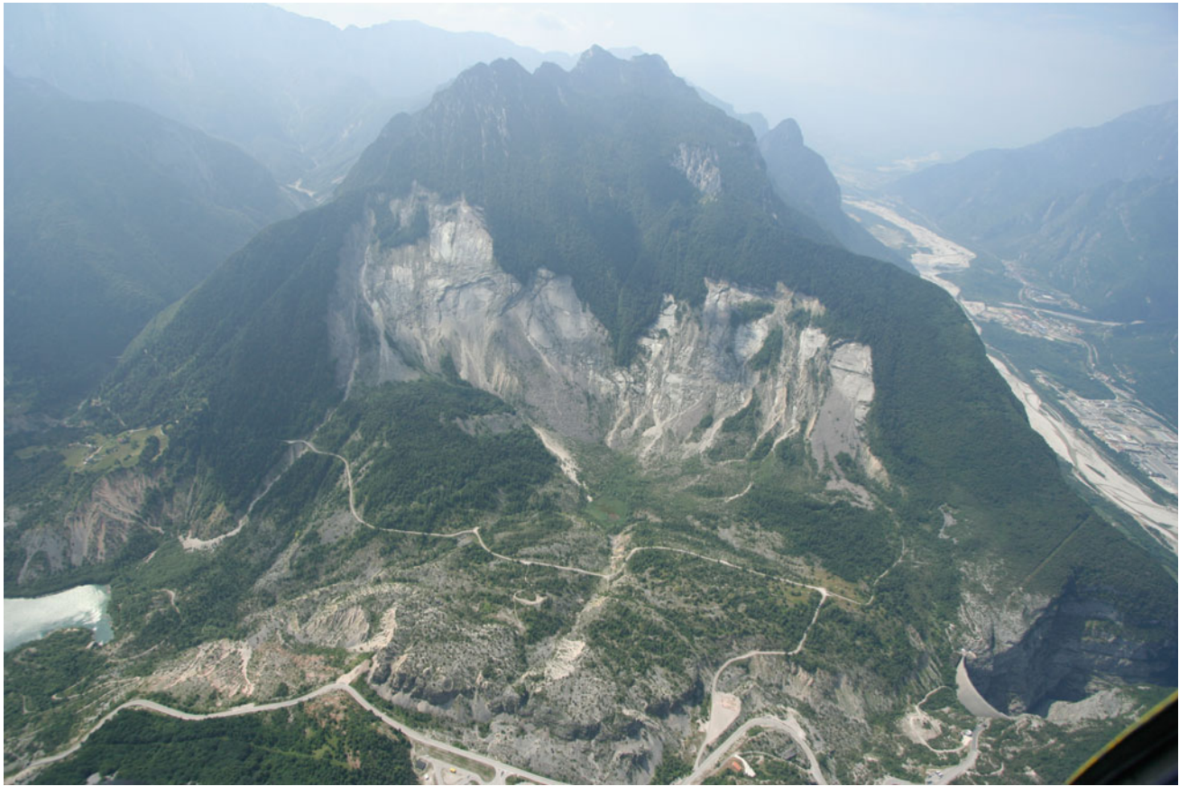
Fig. 11.7 Mt. Toc and Vajont Landslide and dam. The central part of the accumulation zone is characterized by the abandoned valley of Massalezza Stream backtilted toward the sliding surfaces. On the right the Piave River Valley is visible ( photo Virtualgeo)
