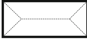
Fig. 5. Single-resolution skeleton graph of a rectangle shape feature
