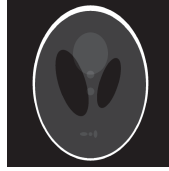
Fig. 2. Standard Shepp-Logan Phantom image.
