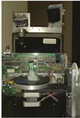
Fig. 1. Optical scanner during the acquisition process of a tooth template.
