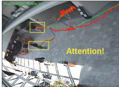
Fig. 5. A logical inference has found a possible case of a sudden attack in the graph of blob trajectories. Rectangle blobs are depicted by yellow lines, blob trajectories are depicted by red lined, moments of interactions between blobs are depicted by green circles and blue links (Color figure online).
