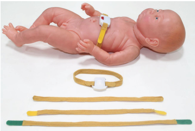
Fig. 6. Prototyped temperature sensor with belts
