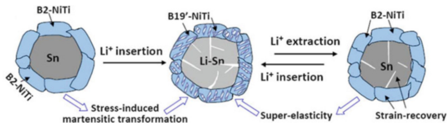
Fig. 4.11 Schematic of morphological changes occurring in Sn–NiTi electrode during charge–discharge cycling. Martensitic transformation ( B2 \rightarrow B19' ) is induced by the stress due to volume expansion of Li insertion into Sn, and this accommodates the stress and strain of Sn. As a result, cracking and pulverizing of the Sn phase is inhibited
