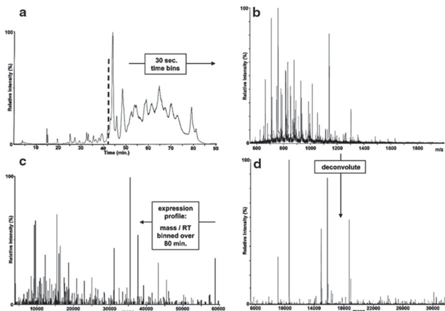
**Fig. 2.7** Generation of protein mass profiles for *Salmonella* spp. using LC-ESI-MS. Multiple-charged signals from proteins within a 30 s time window are deconvoluted into single mass values (mass of neutral protein). The process is repeated for the entire chromatographic period (~80 min) and combined into a single mass profile. (Adapted from McFarland et al. 2014, copyright American Chemical Society)
