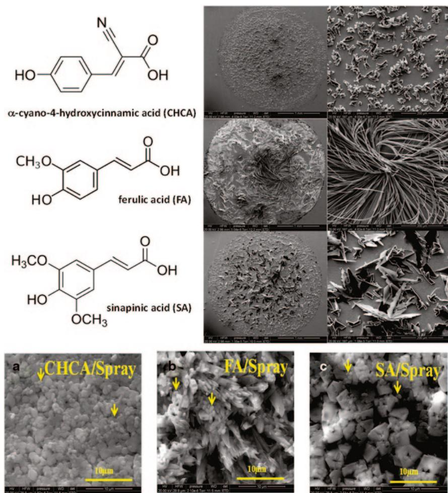
**Fig. 2.2** Structures and scanning electron microscopy (SEM) photographs of different MALDI matrices deposited onto a stainless steel plate. Lower SEM photographs show *E. coli* cells co-crystallized with different MALDI matrices (matrix applied with a spray deposition technique). Arrows point to intact cells within the crystalline matrix. (Adapted from Toh-Boyo et al. 2012, copyright American Chemical Society)
