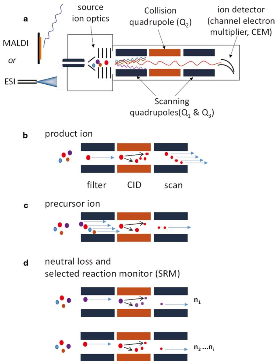
**Fig. 2.4** Triple quadrupole MS, QQQ, where  $Q_1$  and  $Q_3$  indicate scanning quadrupoles and  $Q_2$  indicates the collision cell consisting of either an RF-only quadrupole, hexapole, or octapole. In some hybrid instruments  $Q_3$  is replaced by either a TOF or a linear quadrupole ion trap. (See text for more details and references for further reading)
