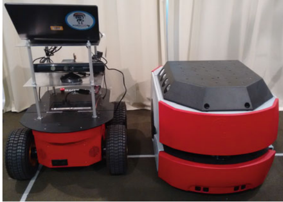
Fig. 1 Side by side are two pioneer ARIA based robots: Pioneer 3-AT and Pioneer LX. These robots, owned by the Advanced Laboratory of Embedded Systems and Robotics of UTFPR, can use the Navigation Stack
