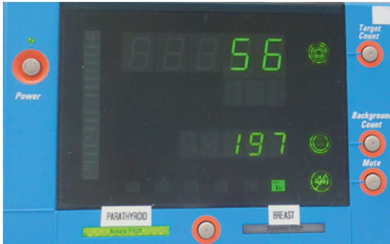
Fig. 13.3 Base unit displaying ratio of target (ex vivo) count over initial background count. In this instance the excised gland measured 28.4 % (56/197), meeting the 20 % rule diagnostic for parathyroid tissue
