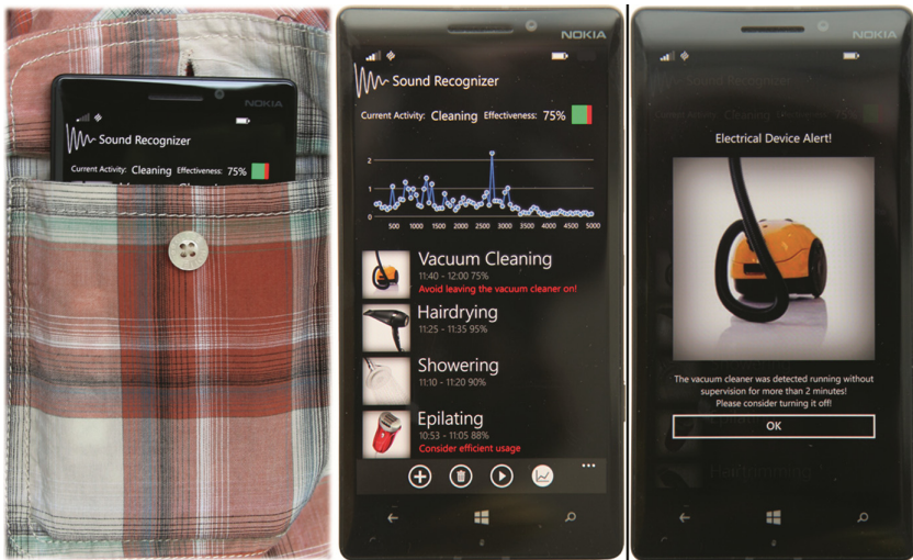
Fig. 3. On-body placement of the smartphone (left) with the application running (middle) and a sample alert (right) after leaving electrical device running longer than desired.
