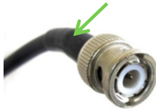
Fig. 6.11 Cable from LDPE filled with \text{Al}_2(\text{OH})_3
