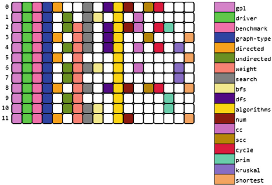
Fig. 2 Graph Product Line 2-wise covering array example [26]
