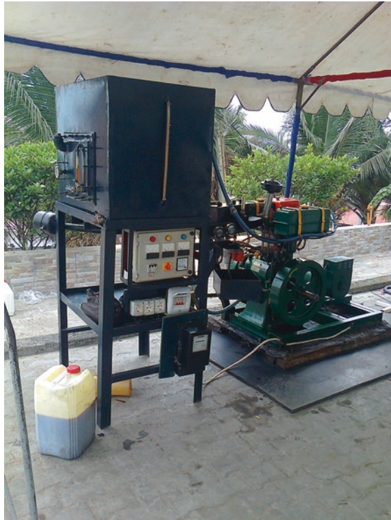
Fig. 1.3 Electric power generator running on crude palm oil
