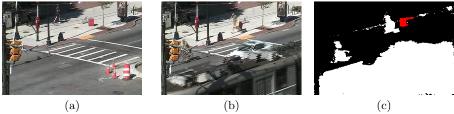
Fig. 3. Example of ghost removal. (a) First image in the sequence, (b) input image from further in the sequence, (c) foreground image, where the removed ghost is denoted in red.
