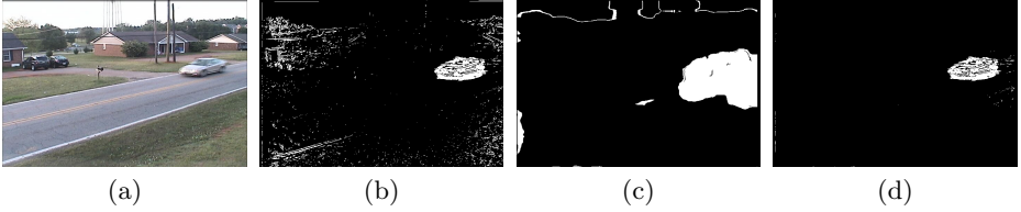
Fig. 4. Creation of the foreground edges in a sequence with panning camera. (a) Input image, (b) Short-term foreground mask, (c) compensated flow mask, (d) logical AND of short-term foreground mask and compensated flow mask.
