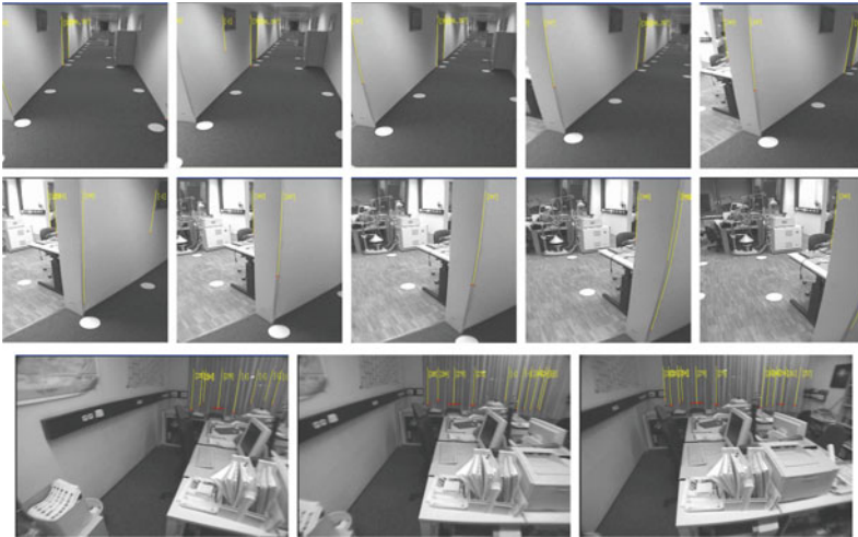
Fig. 5.1 An example of the images used by the 9 robots to test the proposed method [1]. Although the data set also provides artificial landmarks ( white circles on the floor), we do not use them, and instead we test the algorithm using the lines extracted from natural landmarks (in yellow )
