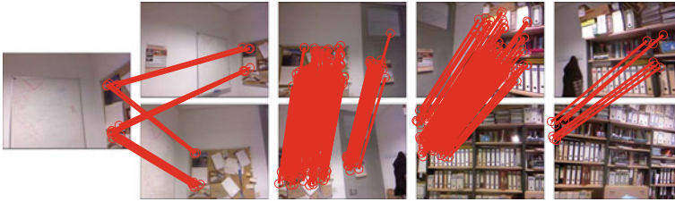
Fig. 5.10 Images taken from the first robot poses. We are depicting the matches ( red lines ) between some of the images
