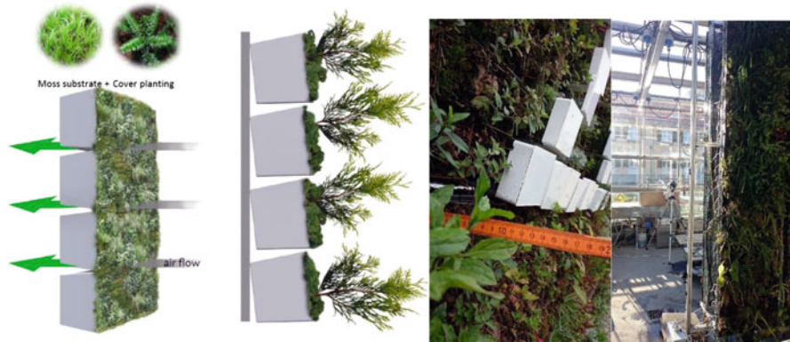
Fig. 6.1 From left to right : Single pot system with moss, plant symbioses, laboratory test for growth, laboratory test of fine dust uptake
