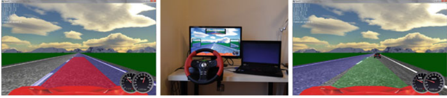
Fig. 5 Example of HMI implementation. The basic setting of driving simulator with integrated driving assistance system ( centre ). The detail of augmented reality-based HMI that is implemented in the driving simulator (braking suggestion on left and lane change to left and acceleration suggestion on right)
