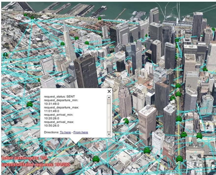
Fig. 4 Simulation run of a taxi-sharing scenario exported in KML format and displayed by Google Earth. The input benchmark was based on historical traffic and demand data from San Francisco, 2008
