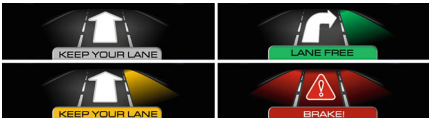
Fig. 3 Examples of visual recommendations of the cooperative driver assistance system
