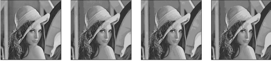
**Fig. 1.** From left to right, the classic lena image ( $512 \times 512$  pixels), its segmented images in eight classes (using seven thresholds) by Otsu (61 87 111 131 148 167 191), Kapur (60 87 112 136 159 180 202) and Kittler (64 89 115 135 149 163 184) methods, respectively.
