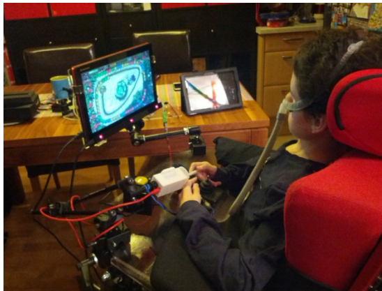
Fig. 5. A 14-year old muscular dystrophy patient using a Tobii EyeX eye tracker and the LipMouse device in combined offset correction mode for desktop control and gaming
