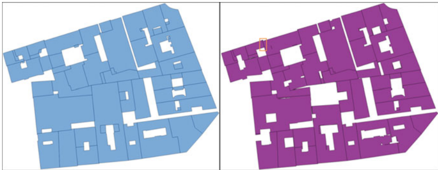
Fig. 11 On the left, cadastral polygons are extended to cover the footprint FP1 extracted from the 3D model. On the right, blue polygons are intersected with FP1 to delete the non-needed part (not present in the 3D model) and obtaining FP3 . The orange rectangle corresponds to a zoomed area used in Fig. 12
