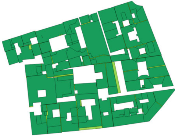
Fig. 13 Split polygons according to 3D discontinuities. Light green ones have been selected for their elongated shape or small area
