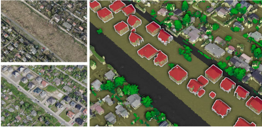
Fig. 2 Multi-temporal 3D point cloud: building points that are not present in the old scan ( upper left ) but captured in the new scan ( lower right ) are highlighted with a red color scheme and by tracing their boundaries
