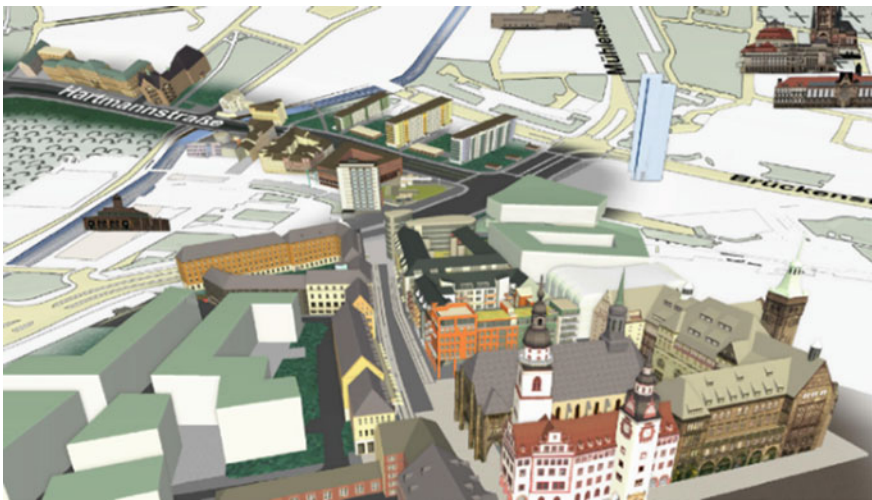
Fig. 12 View-dependent, multi-perspective view and cartography-oriented stylization applied for a route of interest in the city center of Chemnitz. Source (Pasewaldt et al. 2012)
