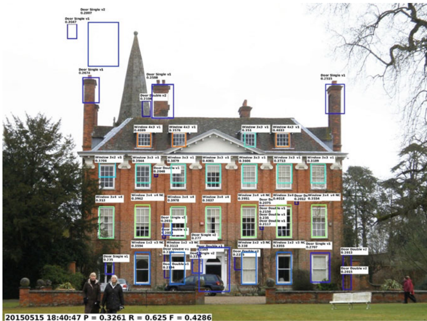
Fig. 5 HOG-based template matching on a Flickr image of Welford Park using multiple templates, bounding box text represents the subclass of the template (line 1) and the ‘match-score’ (line 2)
