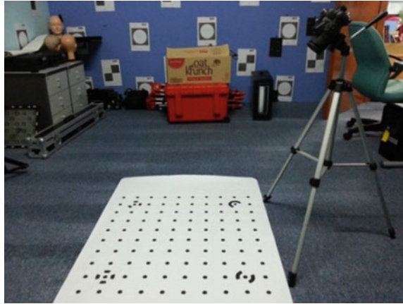
Fig. 2 Photogrammetric camera self-calibration using Photomodeler V5.0 software
