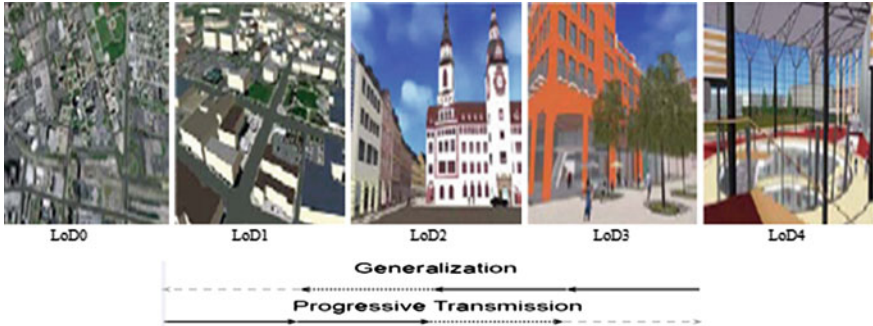
Fig. 4 Multi-scale concept in CityGML (Sester 2007a)
