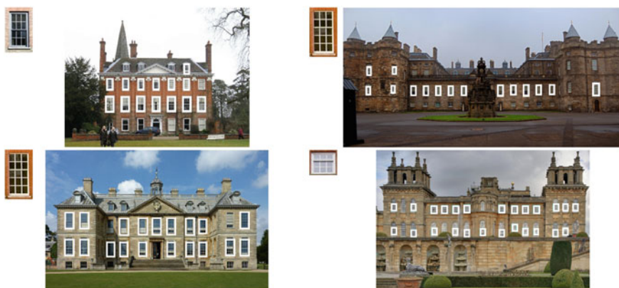
Fig. 3 HOG-based template matching over varying scales on Flickr images of UK heritage properties Welford Park (“Welford Park, Newbury, Berkshire” by Amanda Slater is licensed under CC BY-SA 2.0; Template: from a Google Image Search result) ( top-left ) and Holyrood Palace (“Holyrood palace” by Asif Musthafa is licensed under CC BY-NC-ND 2.0; Template: “IBM Hursley” by Alexis Birkill is licensed under CC BY-NC-SA 2.0) ( top-right ), a Wikipedia image of Belton House (“South facing front to Belton House” by Wehha is licensed under CC BY-SA 3.0; Template: “IBM Hursley” by Alexis Birkill is licensed under CC BY-NC-SA 2.0) ( bottom-left ) and a Flickr image of Blenheim Palace (“Blenheim_Palace: Unprocessed (img_8298_hdr)” by Peter Gawthrop; Template: “Winslow Hall” by Lesley; both licensed under CC BY-NC 2.0) ( bottom-right ). For each image the template used is shown top-left , with matches as thick white bounding boxes
