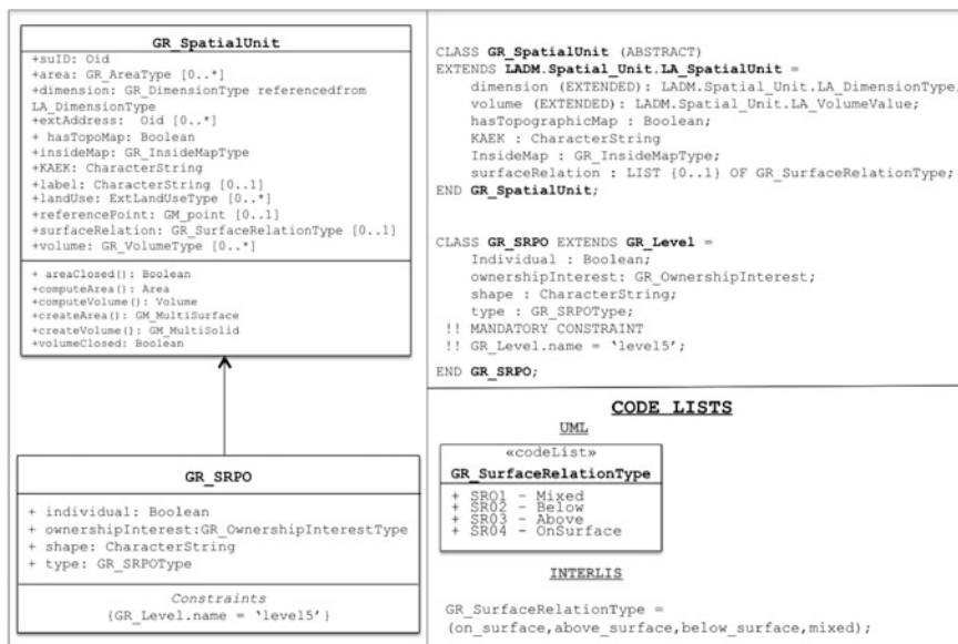
Fig. 8 UML and INTERLIS description of the proposed model
