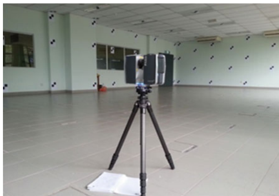
Fig. 1 Self-calibration for the Faro Focus 3D scanner
