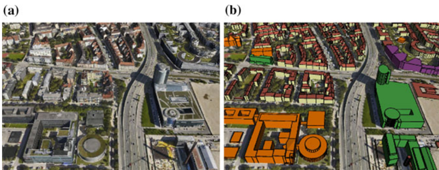
Fig. 5 a A photorealistic visualization compared to non-photorealistic one; b color applied to objects and size applied to edges (Jahnke et al. 2011a)
