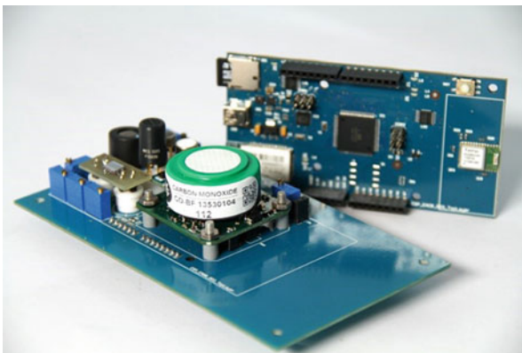
Fig. 7.1 The Arduino board of the sensor box
