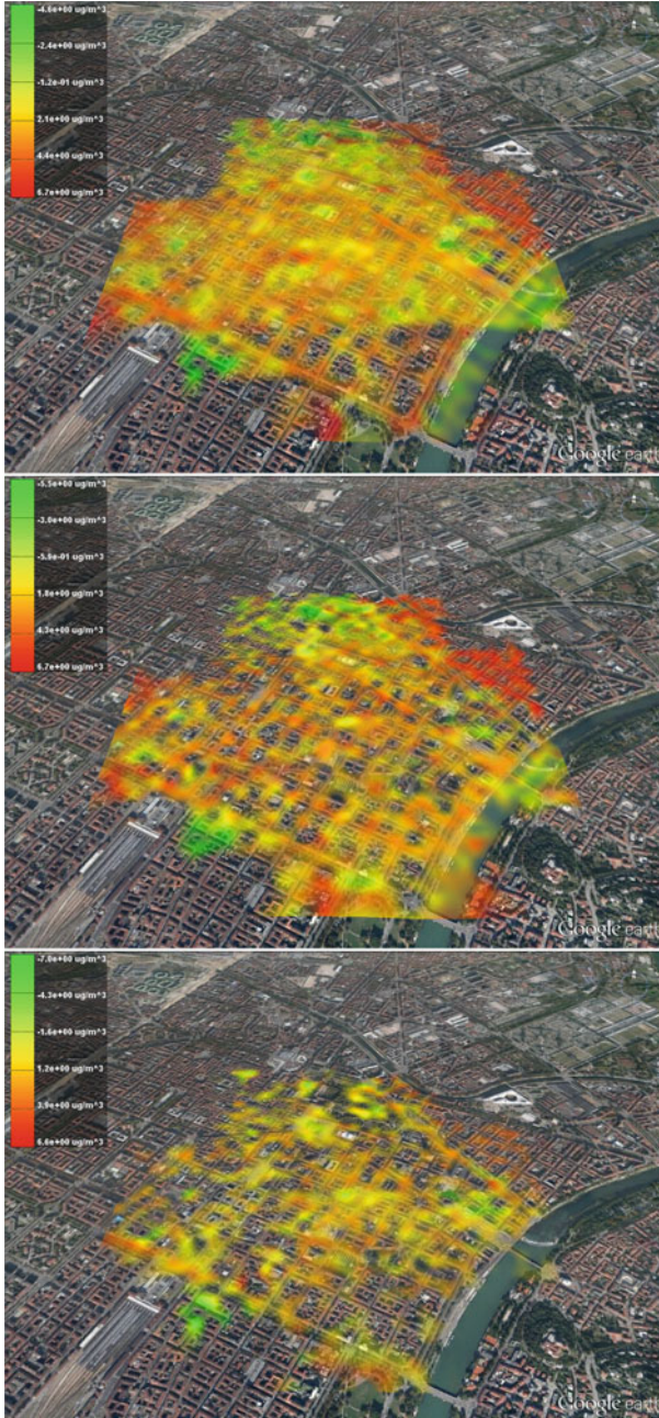
Fig. 16.13 Heat map of the APD values (difference between the web-game annotated AirPin value and the AirSquare value inferred from on field sensor box measurements) for the city of Turin. Top figure refer to phase I, the middle one to phase II, the figure at bottom to phase III. Values in the legends represent \mu\text{g}/\text{m}^3 concentration of Black Carbon. The opacity is related to the number of AirPins used in the corresponding point
