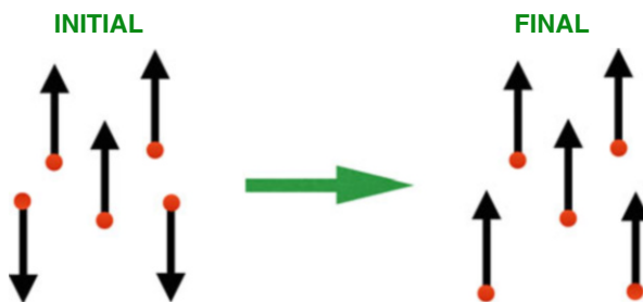
Fig. 17.3 Majority Rule model. The majority opinion inside a discussion group (here of size five) is taken by all agents
