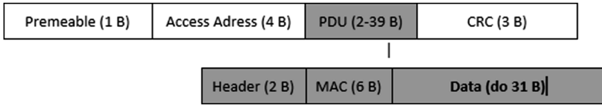
Fig. 1. Packet structure transmitted by iBeacon.
