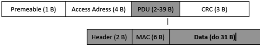
Fig. 1. Packet structure transmitted by iBeacon.
