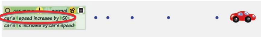
Fig. 8 Increasing the car's speed by a constant amount each tick. This produces a constantly accelerating car
