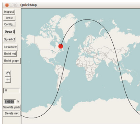
Fig. 2. QuickMap showing an LEO satellite path. This one-period satellite footprint was recorded during approximately 1h and a half. The shift in horizontal position represents the earth rotation during the period.
