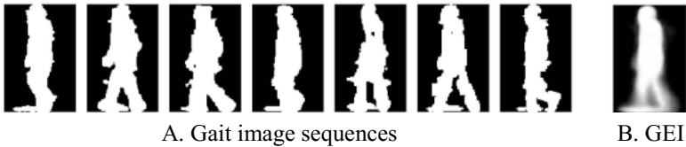
Fig. 1. Gait image sequences of a period and responding GEI
