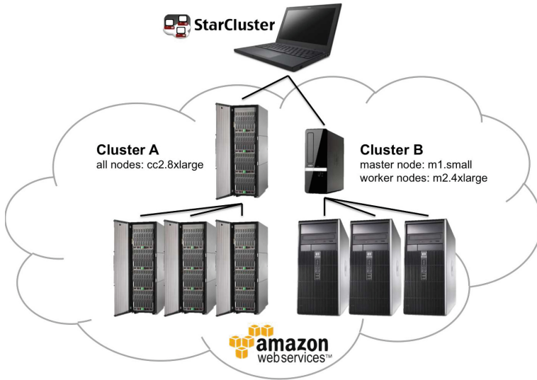
Fig. 2. Examples of both cluster types deployed in Amazon EC2 and used during the experiments.
