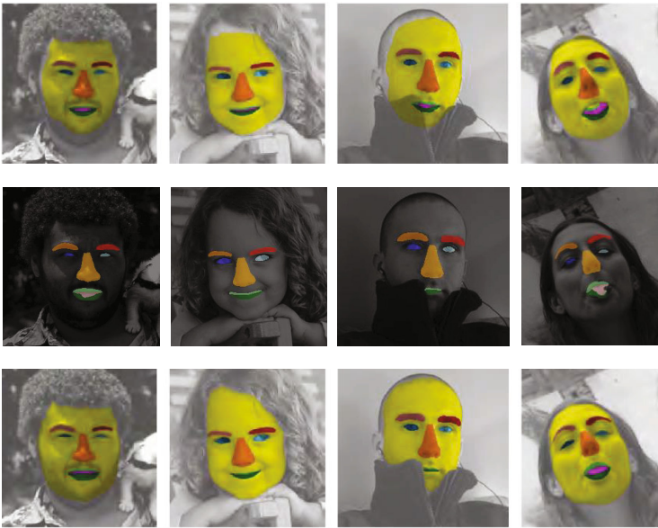
Fig. 4. Labeling results on several example images obtained using the method in [5] (top) and the proposed method in this paper (middle). The bottom shows the ground truth labels. Best viewed in color.
