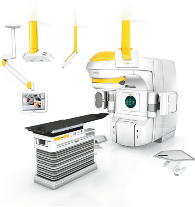
Fig. 14.5 Modern dual photon energy (6 MV and 20 MV) linear accelerator (Novalis TX, manufactured in collaboration between Varian Medical Systems, Palo Alto, CA and BrainLAB, Feldkirchen, Germany) equipped with several imaging modalities for use in image guided radiotherapy (IGRT), adaptive radiotherapy (ART), gated radiotherapy, and stereotactic cranial as well as extracranial radiosurgery. The machine incorporates a high definition multileaf collimator as well as a robotic treatment couch and allows static as well as dynamic intensity modulated treatments. Courtesy of BrainLAB, Feldkirchen, Germany. Reproduced with Permission
