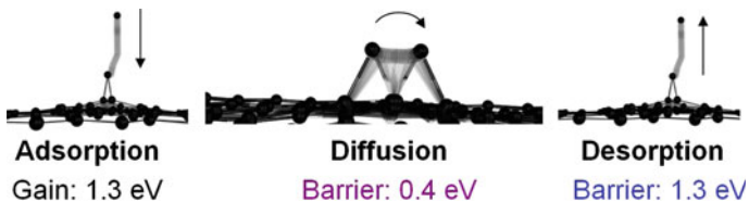
Fig. 8.1 Adsorption, diffusion and desorption of C atoms on graphene. The gray trails connect the initial and final atomic configurations on the NEB/CI reaction path
