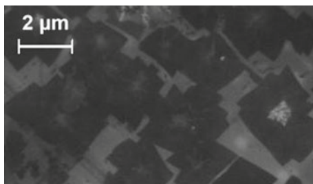
Fig. 8.19 Scanning electron microscope (SEM) image of graphene on a Ge pillar such as that in Fig. 8.18. Black areas are more conducting than the gray areas and are interpreted as graphene flakes. The gray areas may be associated with a more polycrystalline film, possibly with Ge intervening at grain boundaries
