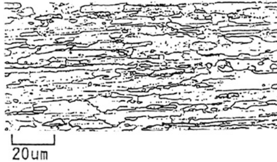
Fig. 3.12 Optical microstructure of cladding tube for F95 steel after second heat treatment (adapted from [86])
